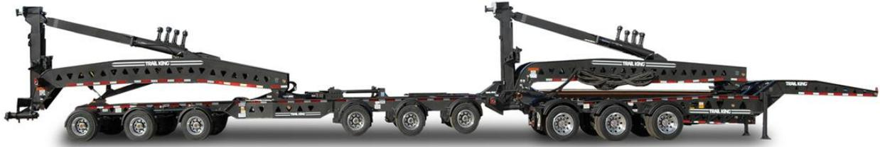
Used to haul wind tower sections, the Trail King Double Schnable trailer consists of a TK100JLW Jeep rated for 100,000 lbs, a Jeep Schnable Gooseneck rated for 85,000 lbs, a TK120LPD-HS Steering Dolly rated at 120,000 lbs, and a Dolly Schnable Gooseneck rated for 85,000 lbs.
