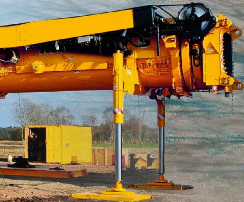
The assembly of the boom on the job site can optionally be carried out without an auxiliary crane. By means of four special support jacks the boom is lifted so that the low bed trailer can move off and the chassis of the LTM 11200-9.1 can be positioned below the boom to the front or the rear. The boom can now be mounted to the chassis with a few manual actions.
