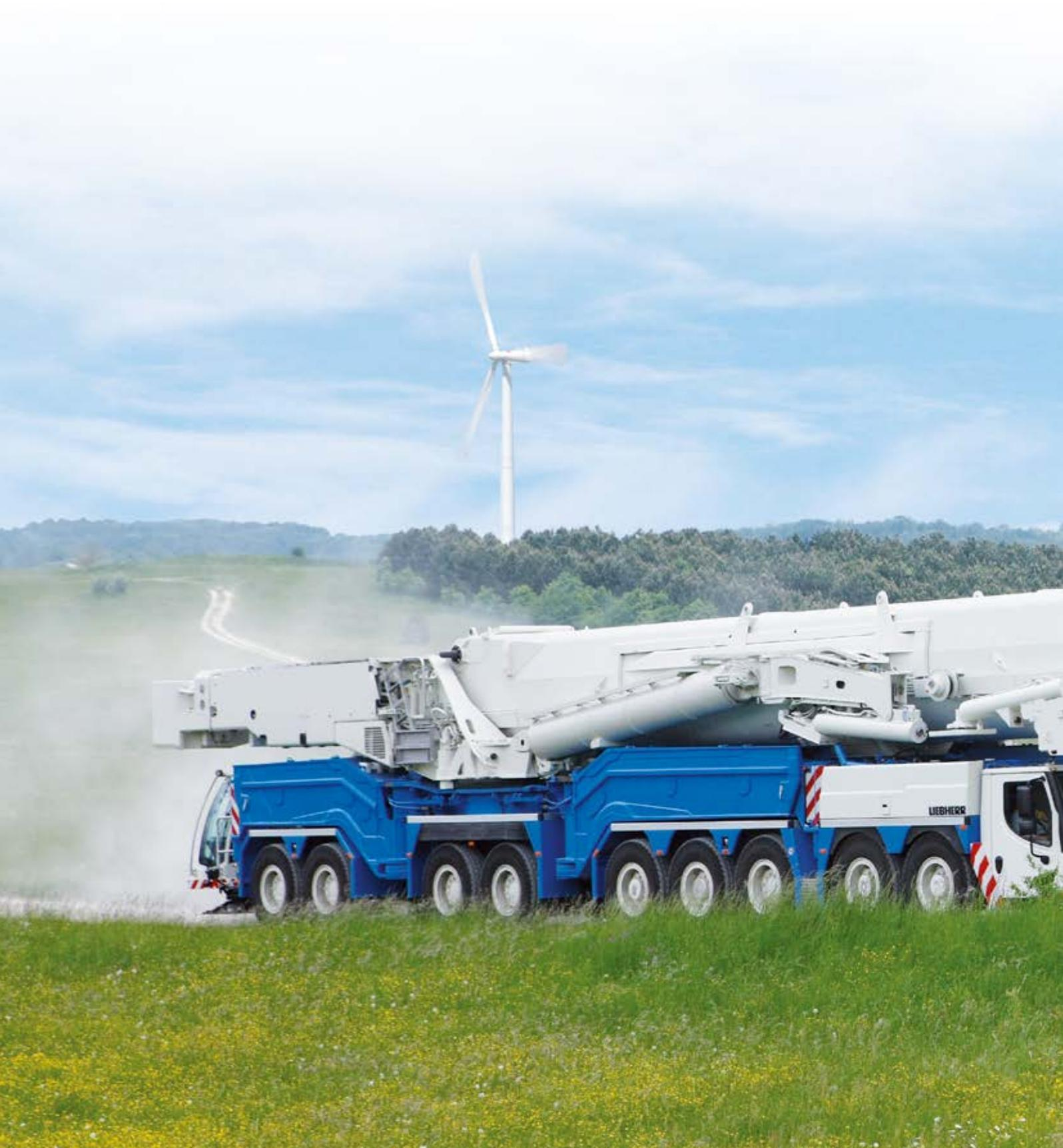
The LTM 11200-9.1 with its capacity of 1,200 t is the strongest telescopic mobile crane in the market and offers the worldwide longest telescopic boom. A remarkable increase of the capacity is realized with the Y-telescopic boom suspension. Short erection times, an extraordinary mobility as well as a comprehensive comfort and safety configuration distinguish the mobile crane LTM 11200-9.1 from Liebherr.
